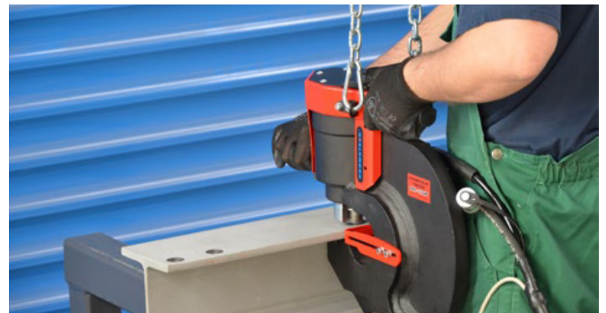
Hoist arm and 2 supports with wheels allow for easy manipulation of punch and power pack as single unit.
