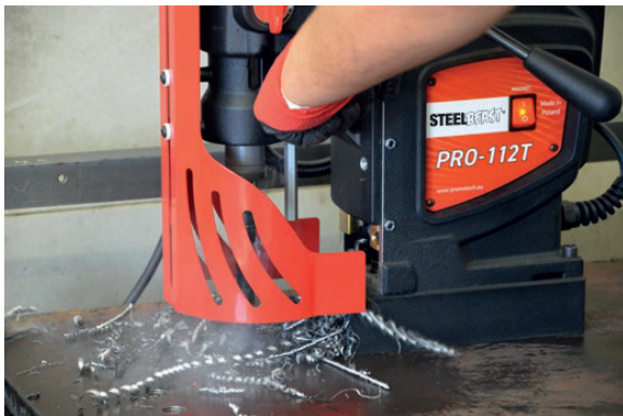
Counterclockwise (CCW) rotation User-friendly control of tapping tool release
